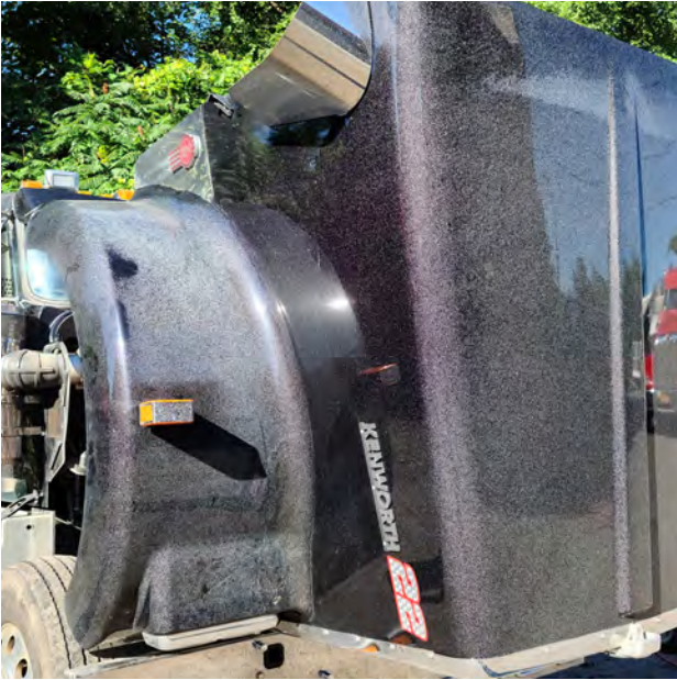
OVERSPRAY DAMAGE (BEFORE)
