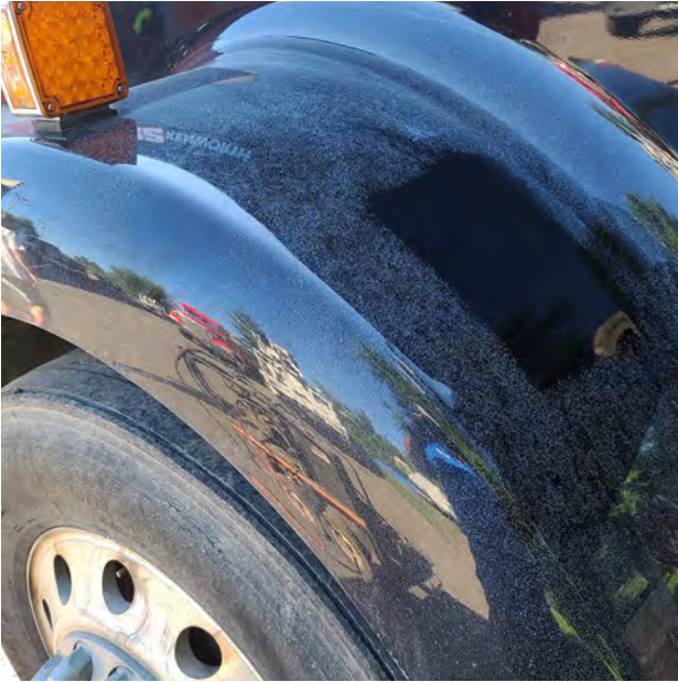
OVERSPRAY DAMAGE (BEFORE)
