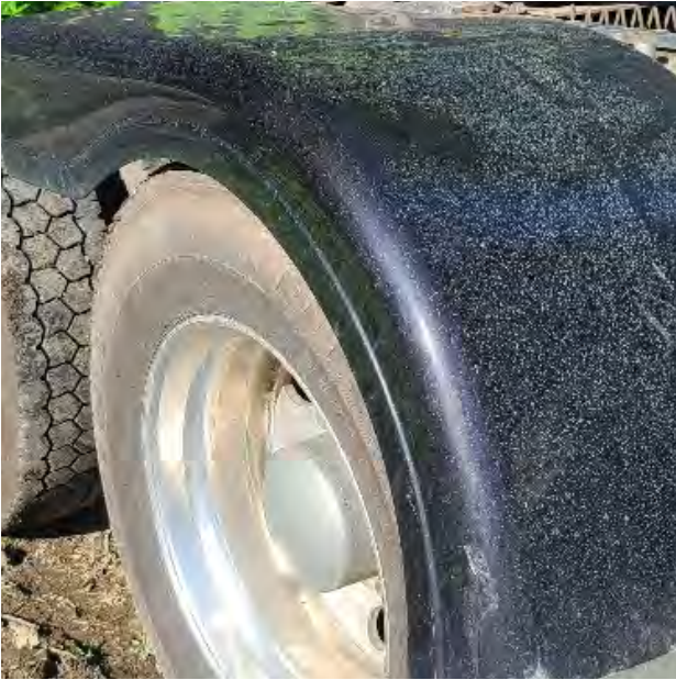
OVERSPRAY DAMAGE (BEFORE)
